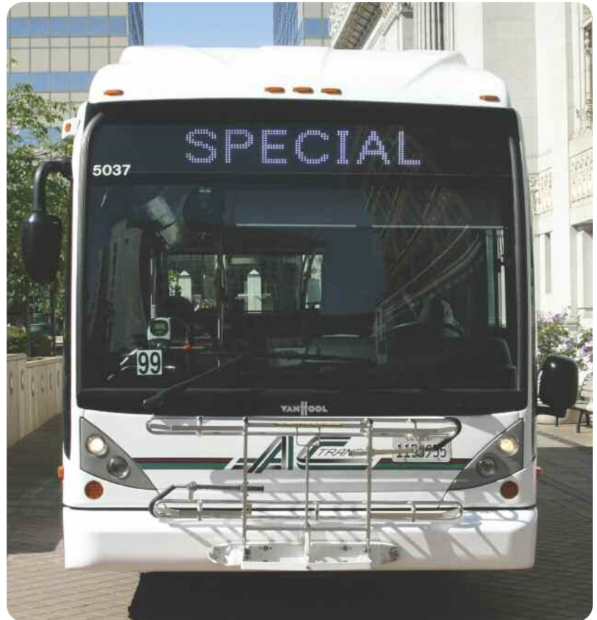
This AC Transit bus in Oakland, California, was built by Van Hool with a Cummins engine. Courtesy AC Transit
